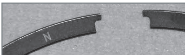
The letter marked on the piston rings.
