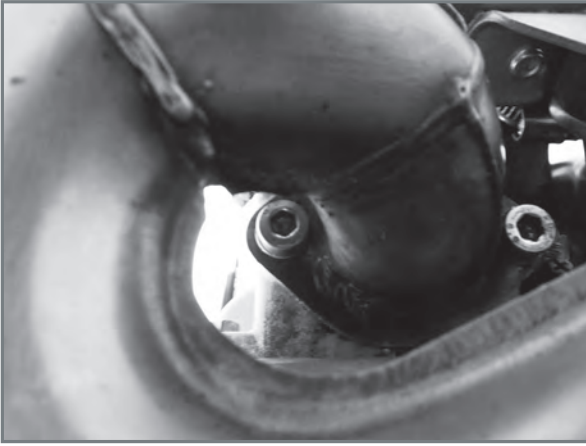
The two bolts of the exhaust manifold flange.
