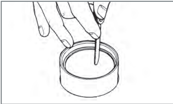
First verification of the piston rings.
