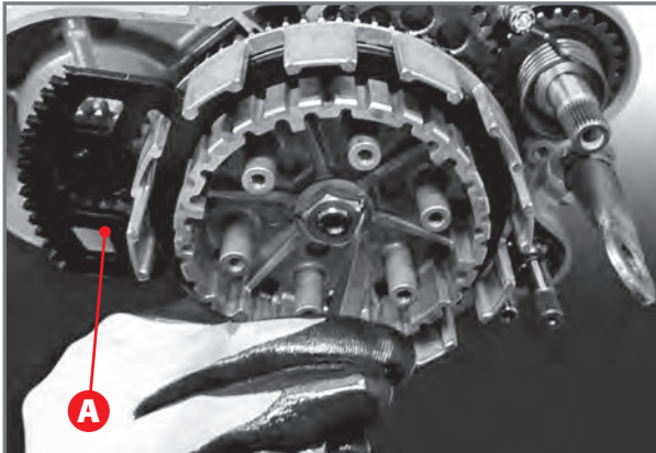
Opening the flaps of the safety washer.
