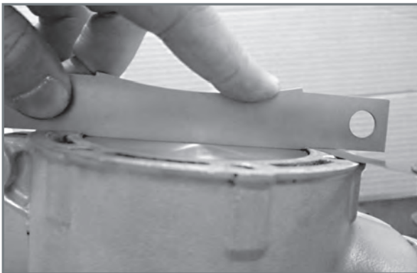
The piston moves the tool on the top.
