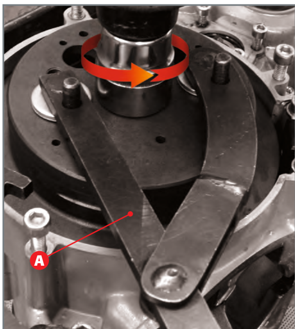
Removal of flywheel nut.
